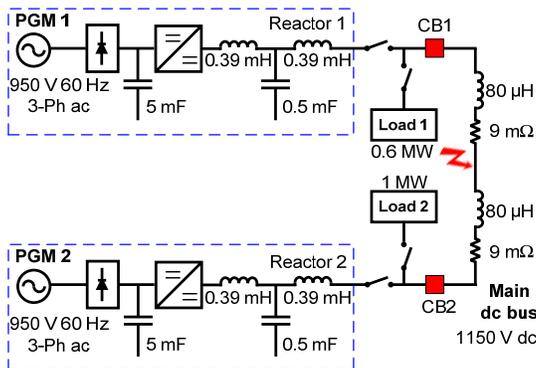
Fig. 4. SLD of the simulated system in Matlab/SIMULINK.
