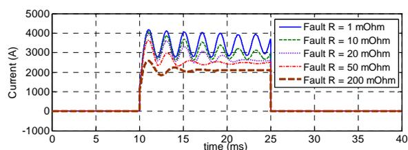
Fig. 6. Current differentials in the main dc bus protection zone with different fault resistances.
