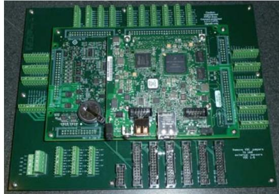
Fig. 9. Capacitor charging power supply control platform.
