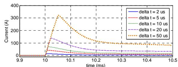
Fig. 7. Current differentials in the main dc bus protection zone with different measurement time differences.
