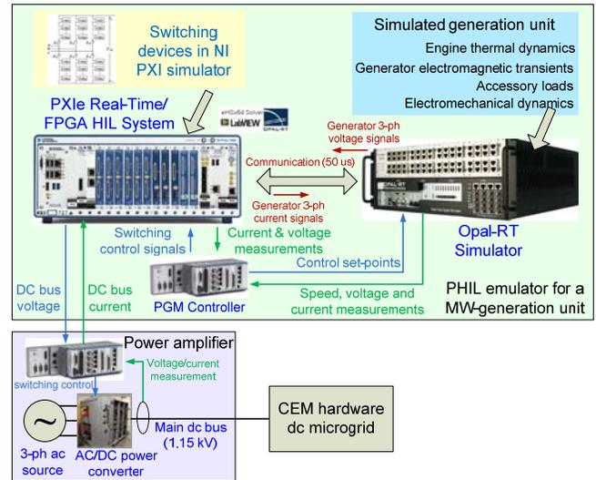
Fig. 13. Diagram of a PHIL emulator for a generation unit.
