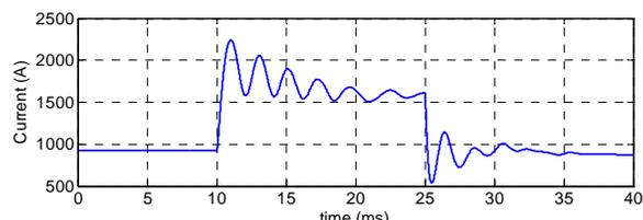
(f) Current flow on the contactor of PGM2
