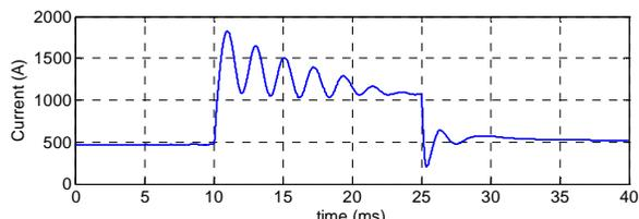
(e) Current flow on the contactor of PGM1
