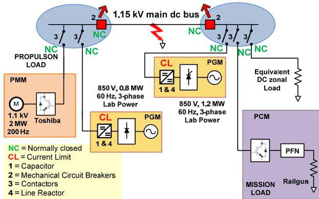
Fig. 2. Diagram of a simplified MVDC system for protection system test.
