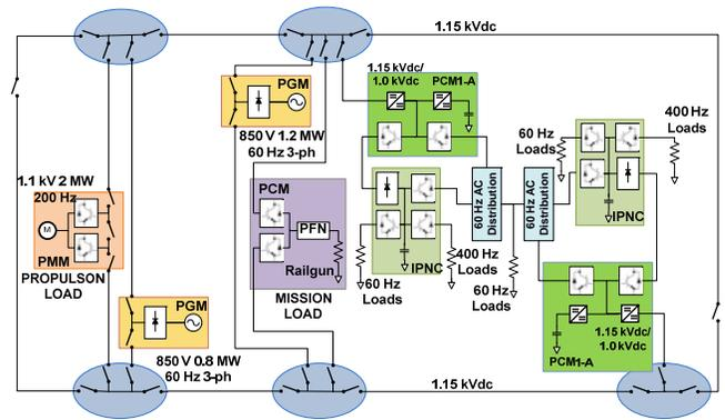
Fig. 1. Configuration of the UT-CEM dc microgrid test-bed.
