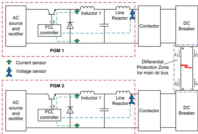
Fig. 3. Diagram of the converter FCL + differential protection scheme.
