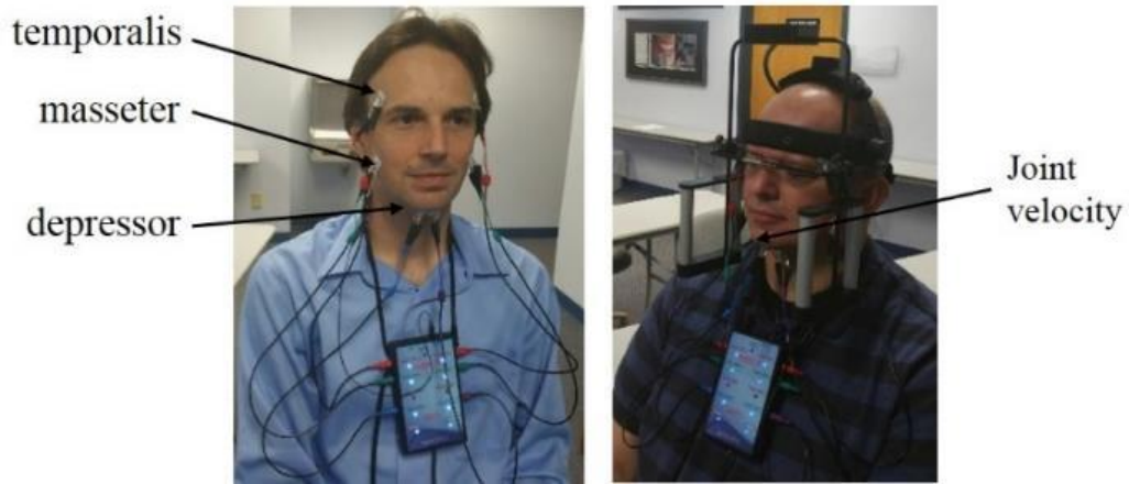
Figure 11. Experiment setup for TMJ cyclic motion data set. The left figure shows the subject involved in the experiment, while the right figure presents the magnet-based 3D jaw tracker
