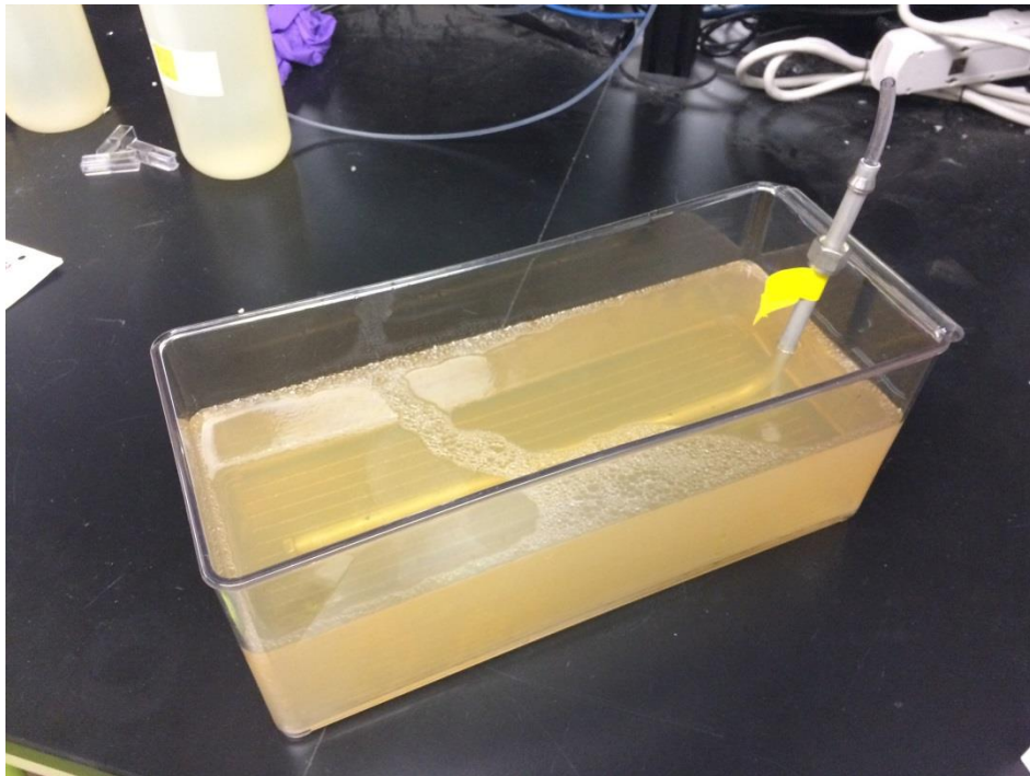
Figure 3.3c – Cured gelatin with wellbore inside the container.
