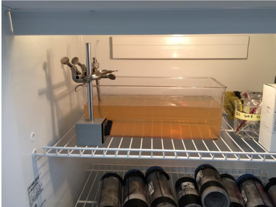
Figure 3.3b – Container with wellbore with gelatin placed in the refrigerator for curing.
