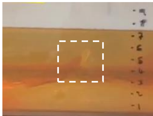
Figure 4.2 – Fracture growth with the air previously present in the wellbore at the crack tip, followed by glycerin fracturing fluid. Inside the dotted box, we see the dry tip of the fracture.
