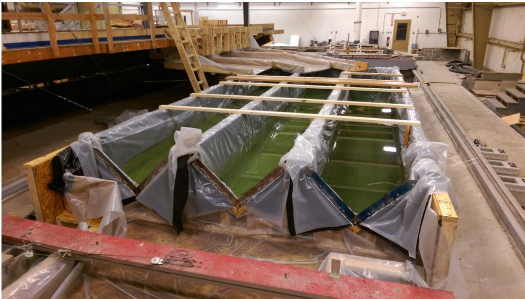
Figure 19. V-notch weirs and approach channels.
