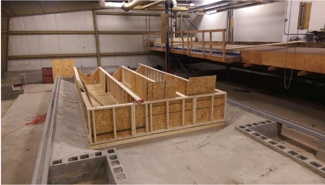
Figure 55. Photo of approach channels under construction.
