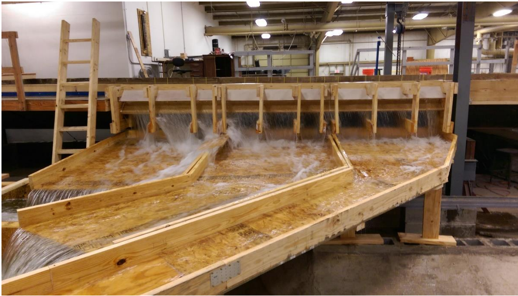
Figure 53. Physical model flumes, directing curb inlet intercepted flow into V-notch weir approach channels (when slab supports are installed, a division of flow between sections is achieved through vertical flow dividers).
