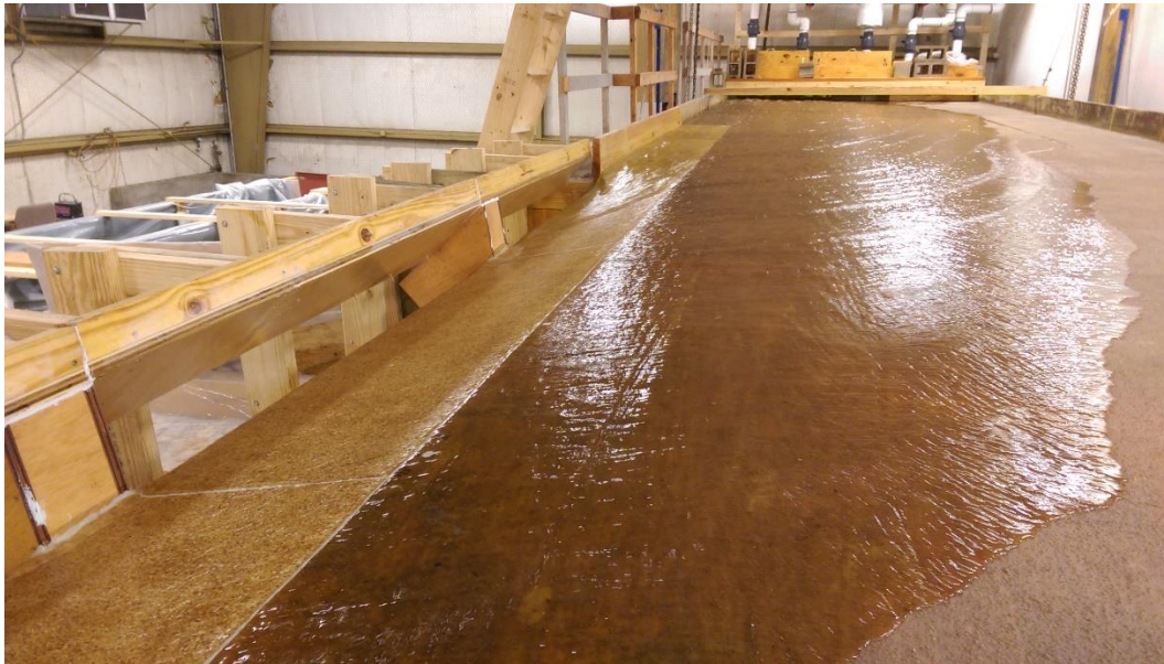
Figure 35. Thin water depth observations on the road surface and gutter section during a 100% interception test for a 15 ft TxDOT curb inlet at S_L=2\% , S_X=2\% (Test #57, Appendix B).
