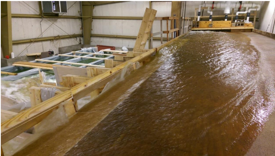
Figure 26. Photo of waves around both internal slab supports for a 15 ft curb inlet at S_L=1\% , S_X=6\% , bypass condition (Test #60, Appendix B).
