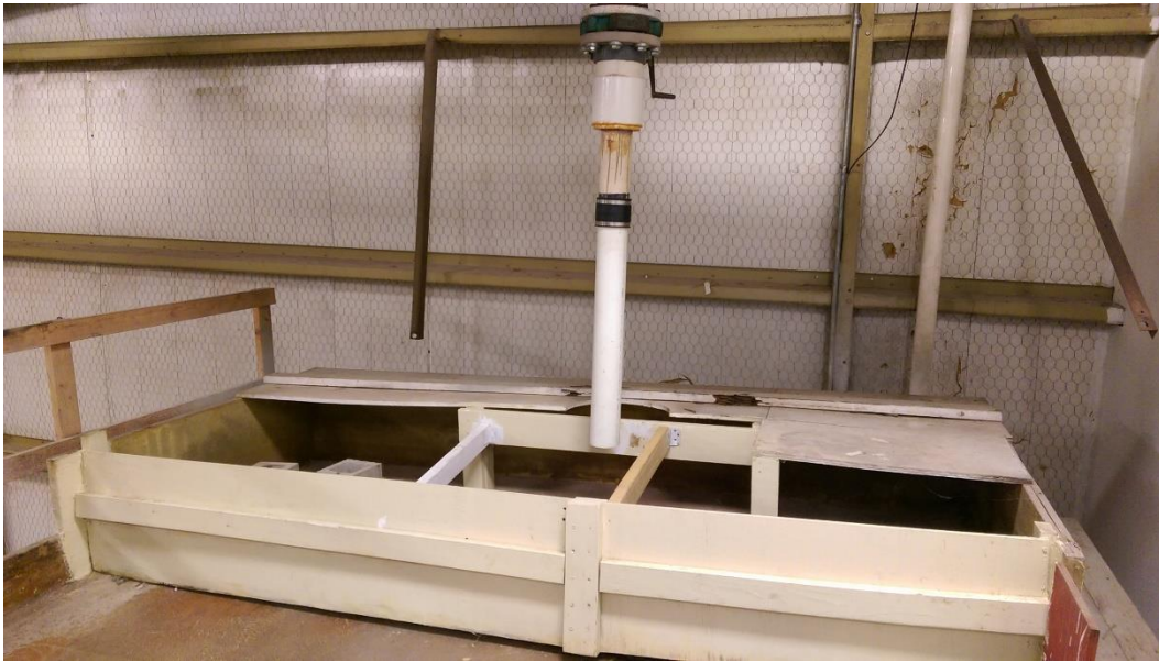
Figure 59. Headbox and inlet pipe before modifications.
