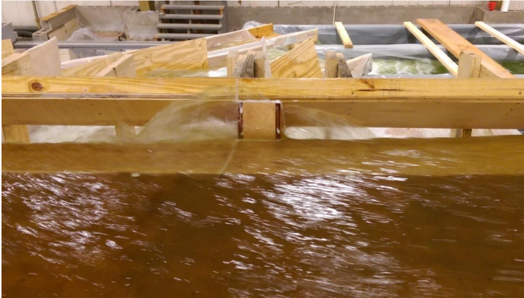
Figure 25. Photo of waves before and after an internal slab support for a 15 ft curb inlet at S_L=1\% , S_X=6\% , bypass condition (Test #60, Appendix B).
