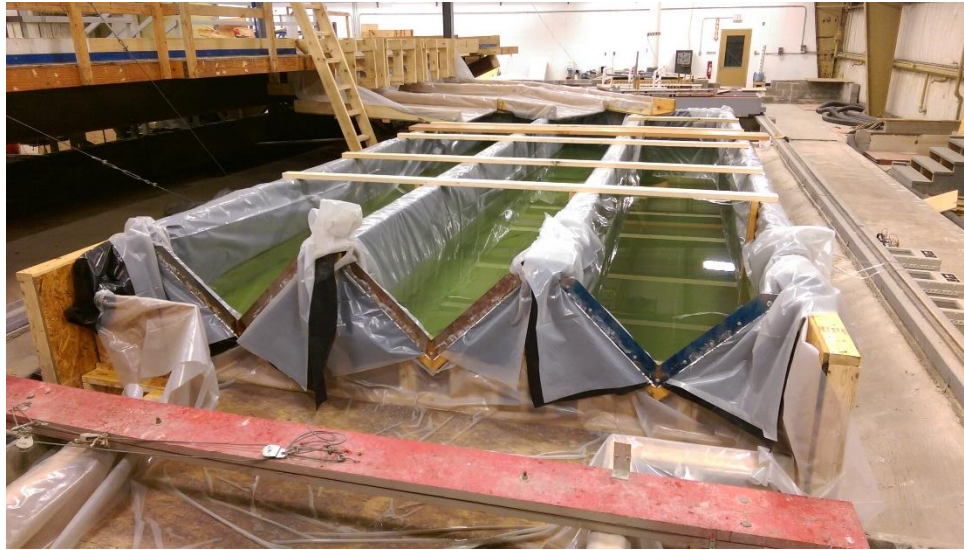
Figure 47. Photo of three 90 degree v-notch weirs and their approach channels with the physical model on the left side of the photo.
