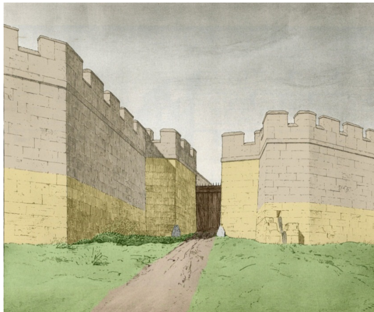
Figure 40 Reconstruction of the Porta Nola during the limestone phase. The color differentiation shows the extent of the tufa addition, after Krischen, Die Stadtmauern von Pompeji , Pl. IV modified by author.
