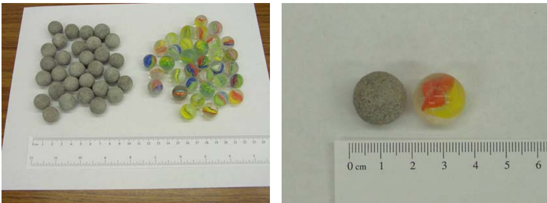
Figure 5.7 Uncoated and coated (smooth and rough) marble
