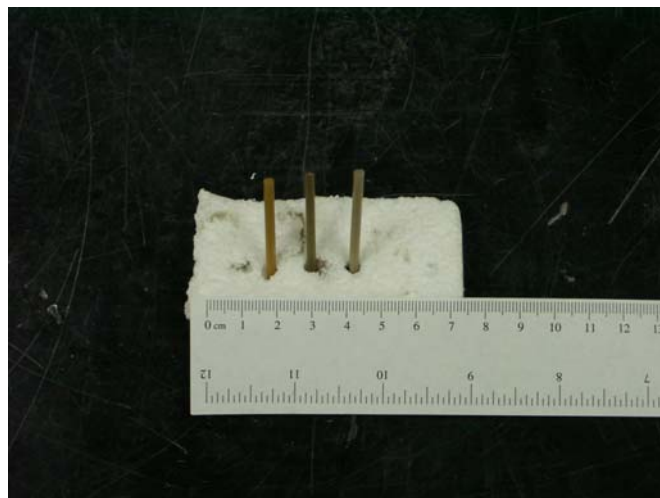
Figure 3.7 Three different microfine aggregate \mu\text{CT} specimens (The top scale bar shows centimeters)
