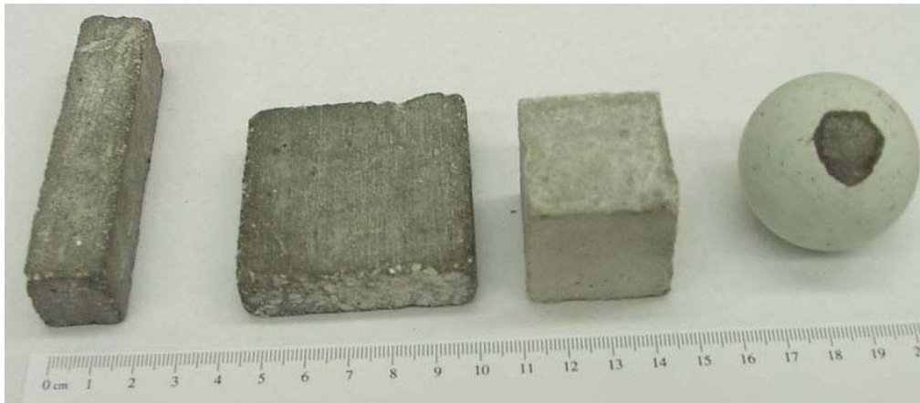
Figure 5.4 The four artificial coarse aggregate shapes
