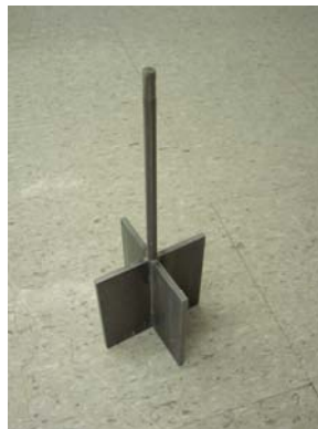
Figure 2.13 Vane impeller used in the rheometer
