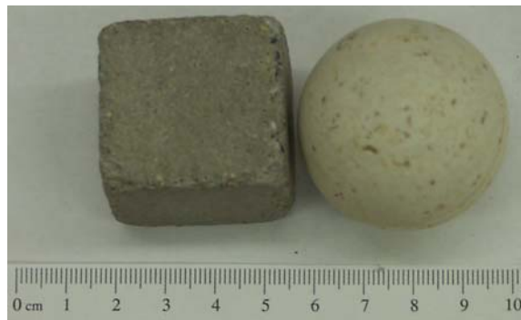
Figure 5.5 The smoothened and roughened surfaces of a sphere and a cube after trial mixtures
