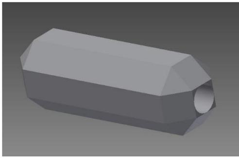
**FIGURE 2 EXTRUDED, CHAMFER, HOLE COMMANDS USED**
