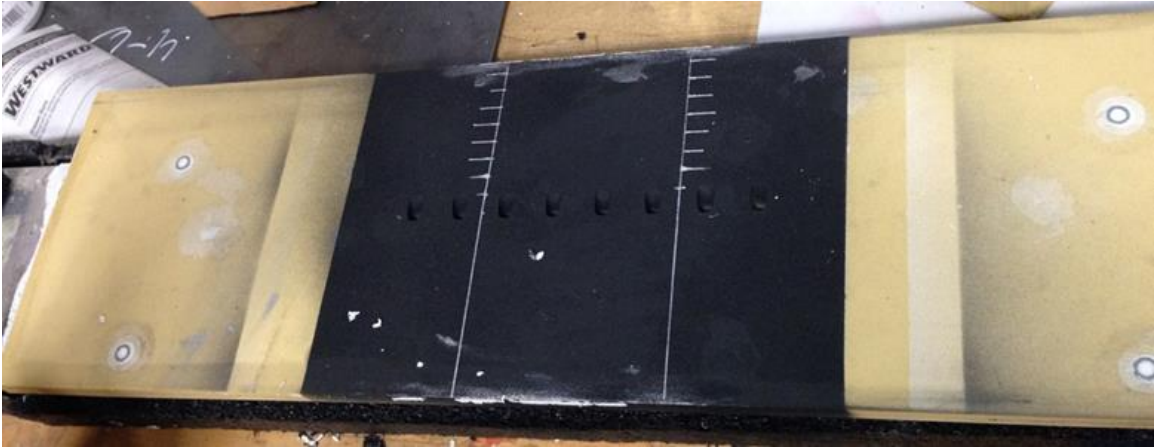
Figure 12: Photo of the 8x scale polyurethane foam coupon assembled to coolant channel
