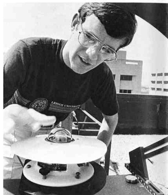
Working on a project to measure Austin solar and wind energy patterns, engineering graduate student Michael Mickalonis adjusts a device that senses diffuse solar radiation.
