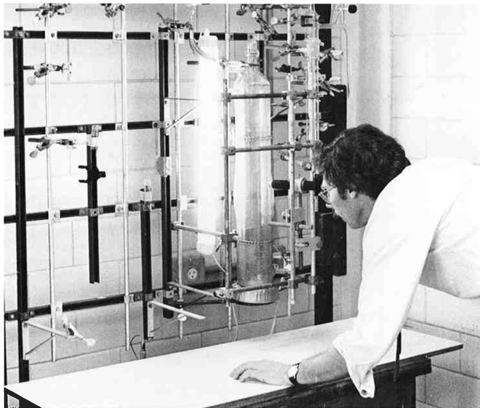
Prof. William Koros, a separations researcher, studies the properties of ultrathin polymer membranes. Some membranes block certain gases or liquids while allowing others to pass through freely. Chemical separation with membranes is a rapidly growing technology that consumes little energy.
