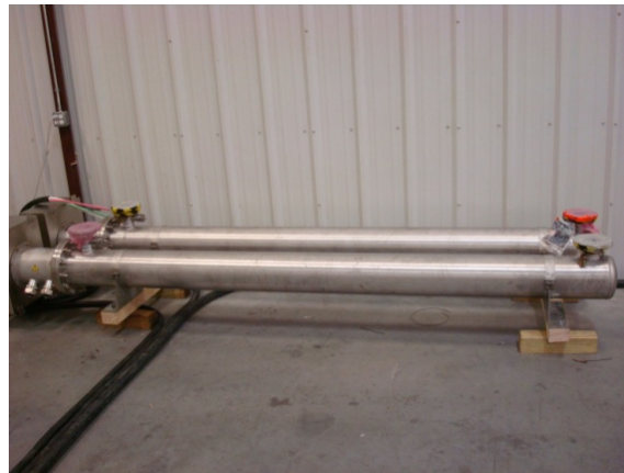
Fig. 2.10 Example of Water Cooled Power Resistor for Power Dissipation
