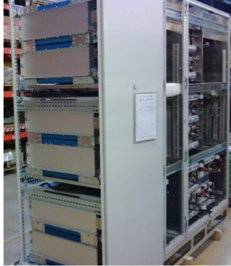
Fig. 2.7 Example of Ultra-Capacitor Banks for Energy Storage System
