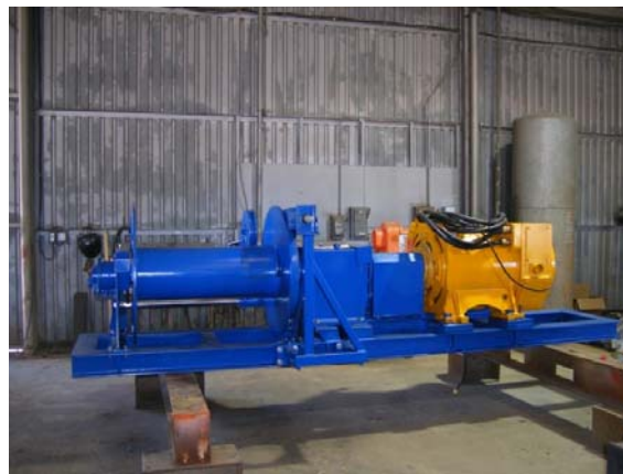
Fig. 2.3 Motor Driven Electrical Winch System with Gearbox
