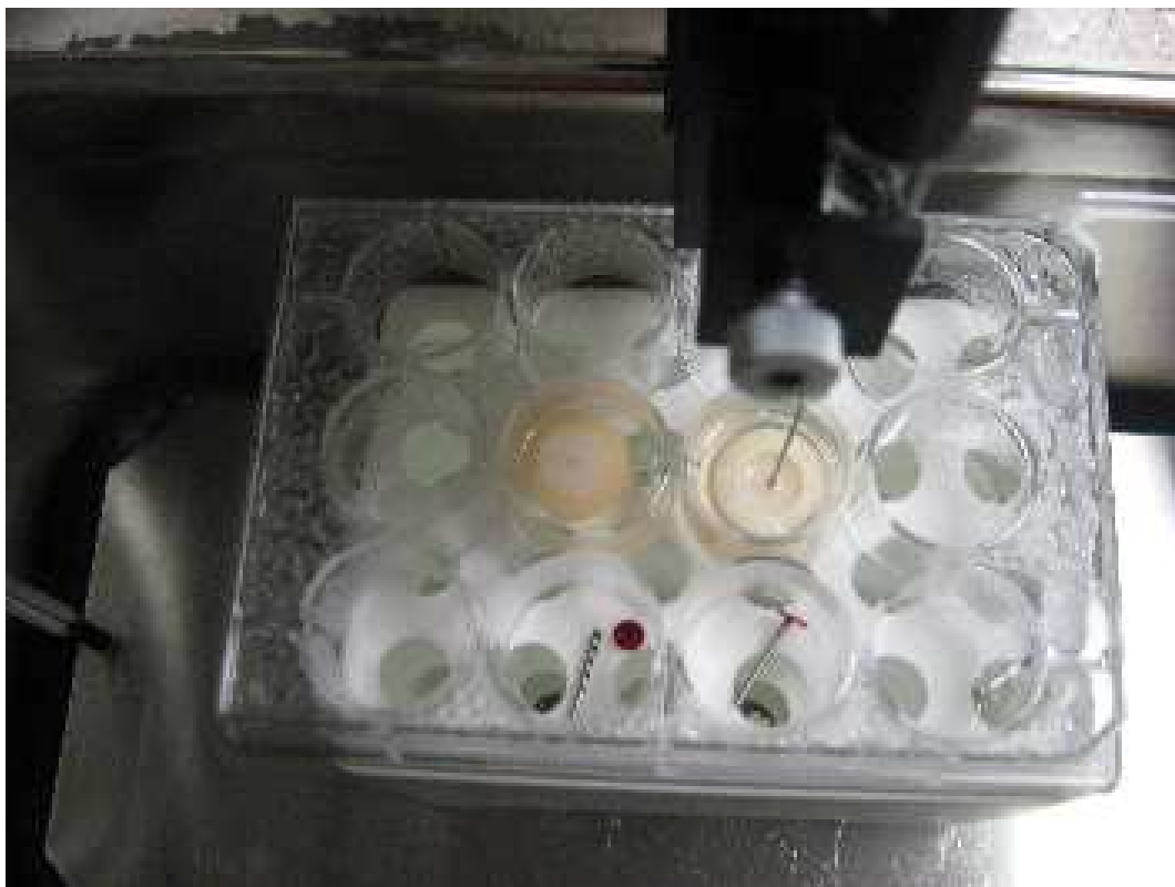
Figure 13. Hypodermic needle surrounding the sensor being descended into the construct.
