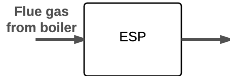
Figure 2.10: After exiting the boiler, the flue gas goes through an electrostatic precipitator, ESP, where fine solid particles are removed.
