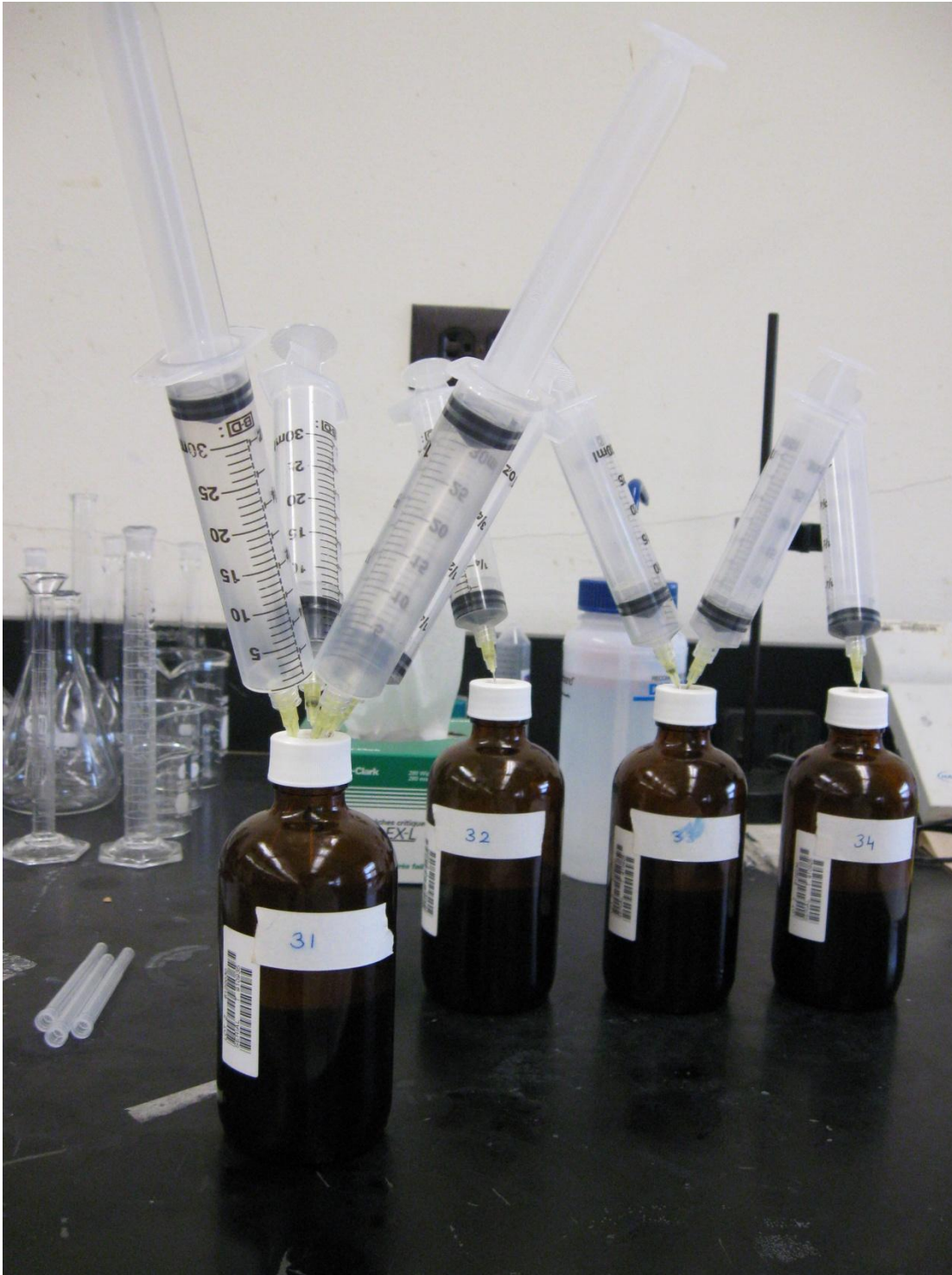
Figure A.2: Biogas measurement from batch digestion bottles.
