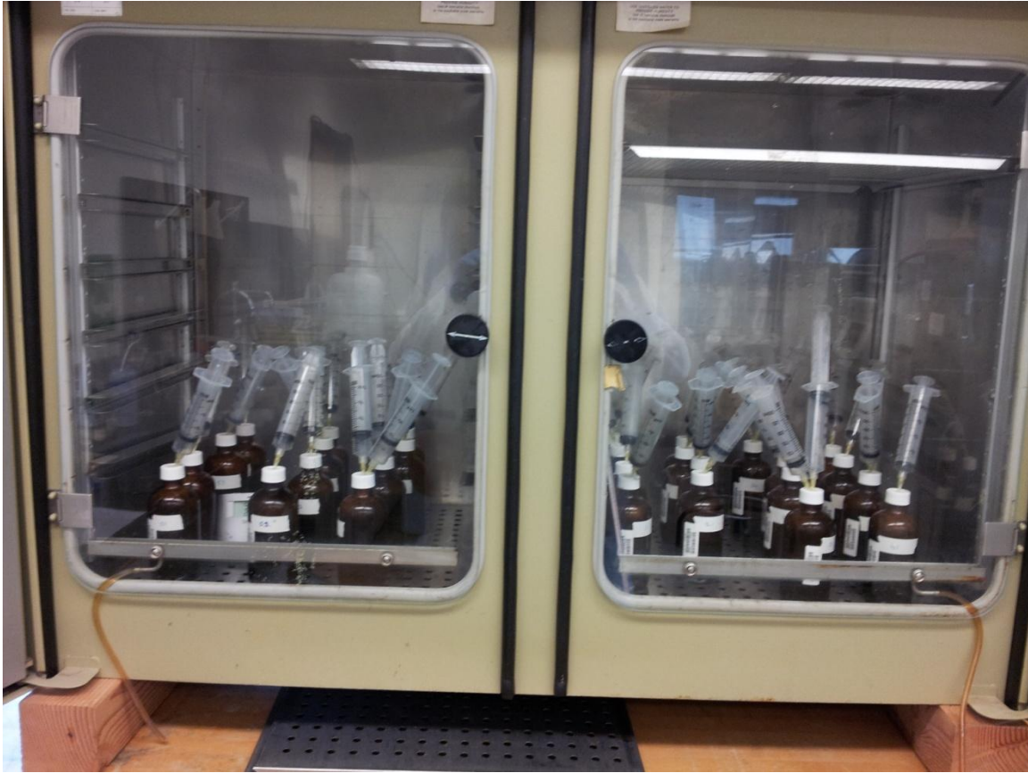
Figure A.1: Batch digestion bottles in the incubator (35 °C).
