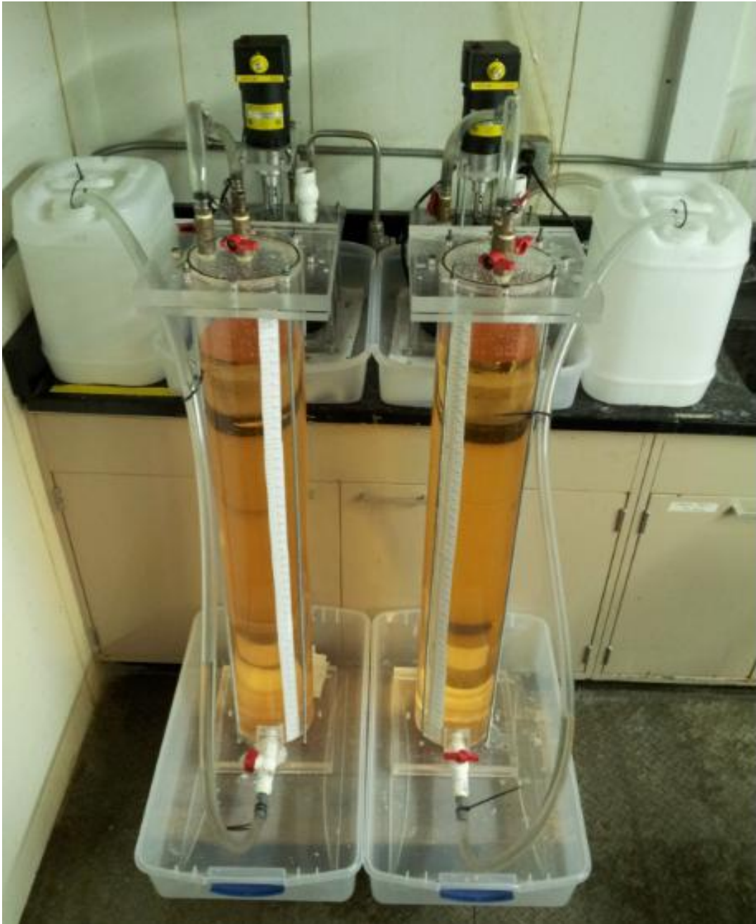
Figure A.3: Anaerobic digestion system, Front-View.
