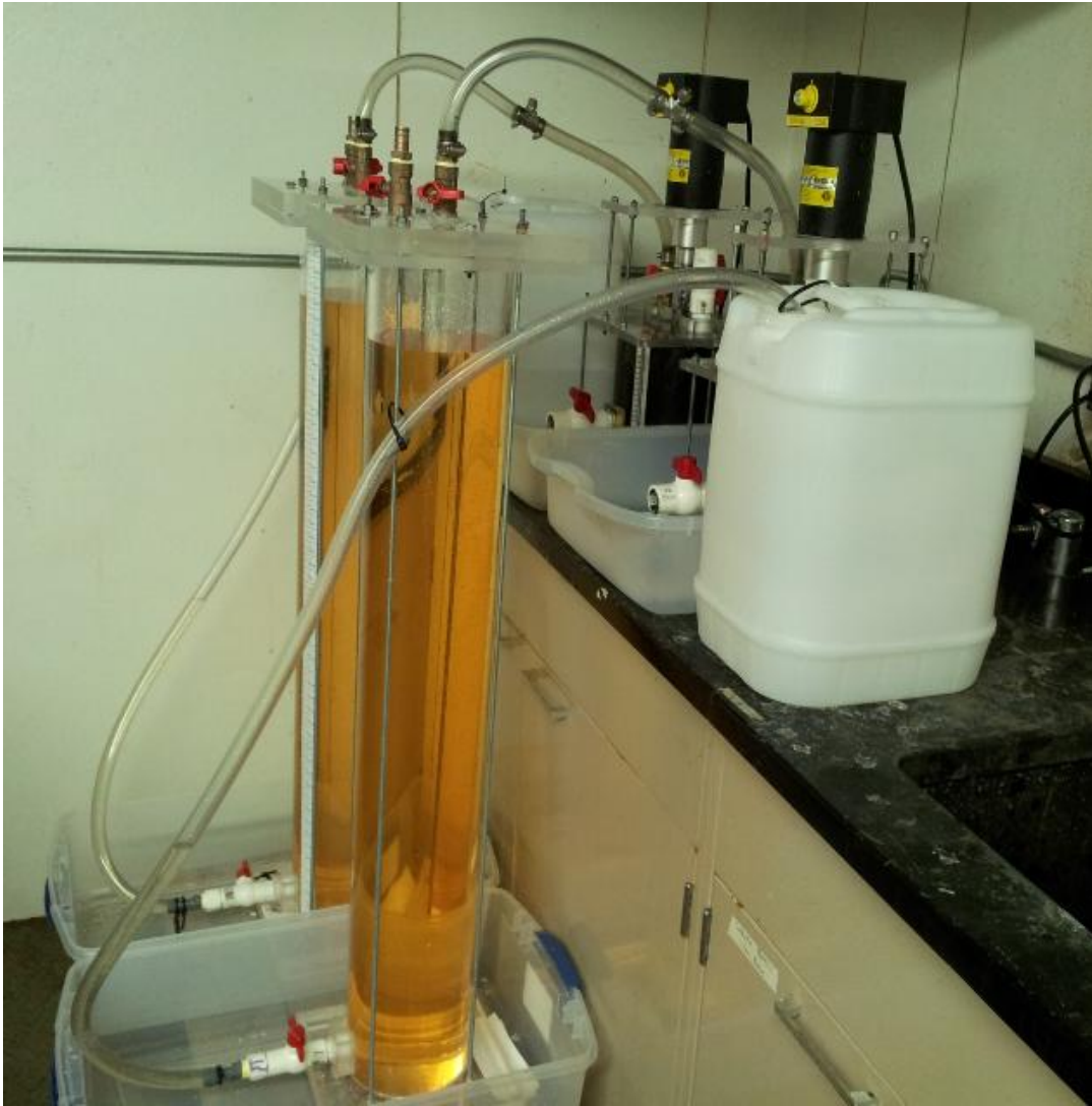
Figure A.4: Anaerobic digestion system, Side-View.
