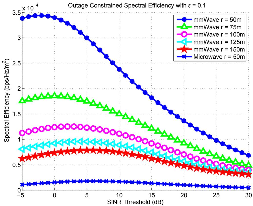
Figure 5.5: Area spectral efficiency of network with 10% outage.
