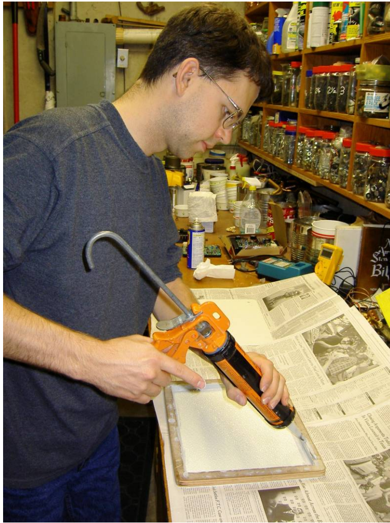
Figure 6.16: Applying Adhesive Caulk to the PersonaWarmth Prototype
