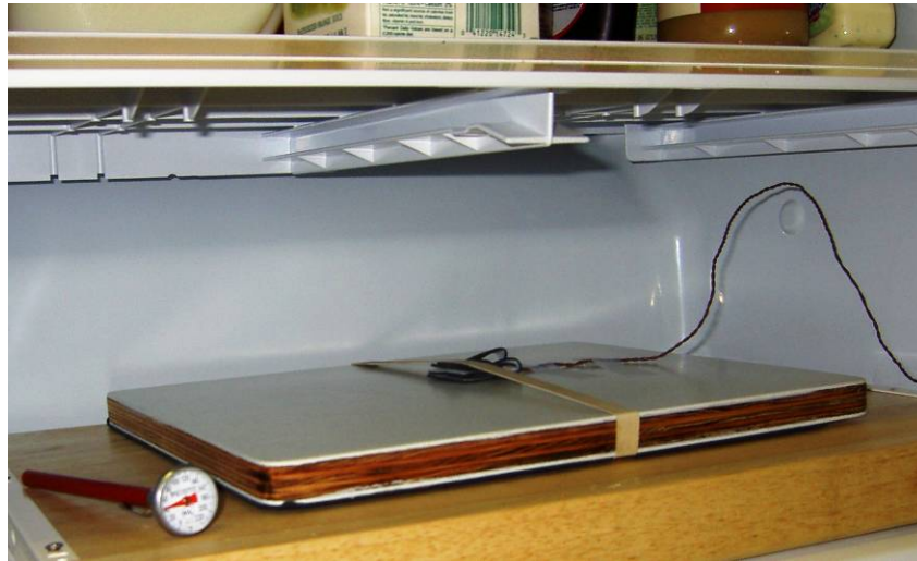
Figure 6.17: Prototype Testing in a ~50°F Refrigerator Compartment
