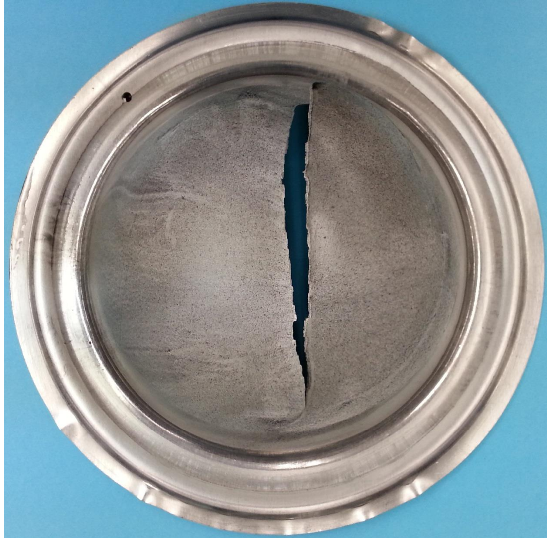
Figure 4.9 Test specimen for Exp. BU12 after failure.
