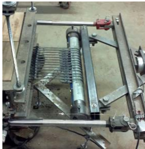
Figure 3.13: Clamping mechanism in the rotated, as-tested state.
