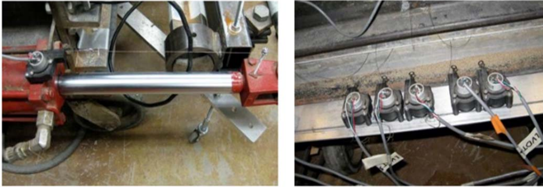
Figure 3.14: LVDTs mounted on a hydraulic piston and at the back of the pull-out box.
