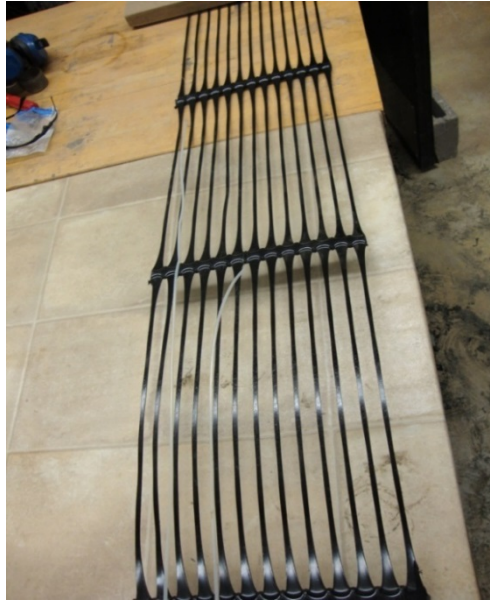
Figure 3.11: Geogrid specimen with attached tell-tales and high strength tubing.
