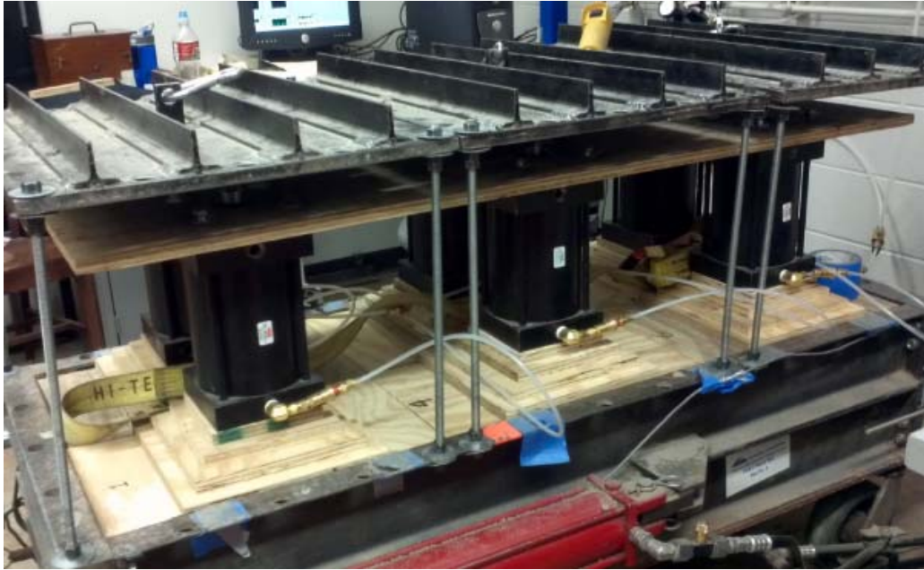
Figure 3.18: Test setup with reaction plates secured over the air cylinders.
