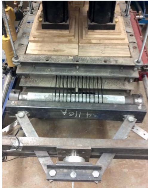
Figure 3.8: Clamping mechanism of the geogrid with a centered load cell.
