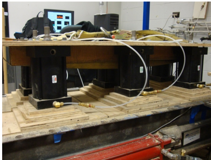
Figure 3.17: Air cylinders atop the plywood pyramids.
