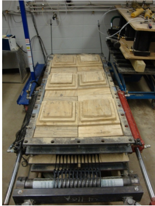
Figure 3.16: Plywood pyramid configuration.
