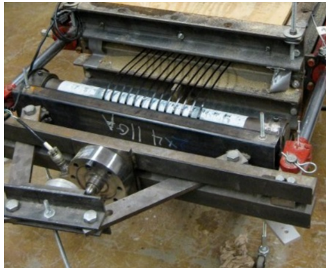
Figure 3.9: Clamping mechanism with load cell detail; prior to the start of a test.
