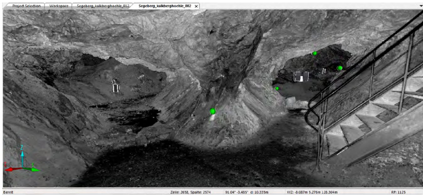
Figure 2. 3D scan of a solutional passage of the Segeberger Kalkberghöhle in anhydrite with typical sloping sidewalls and horizontal ceilings characteristic of a cave created by internal convection.
