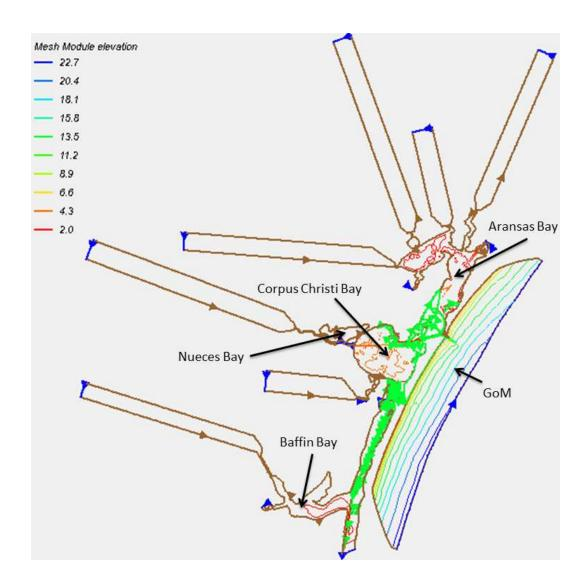
Figure 3.4.1: SELFE grid domain outline. The large rectangular sections are dummy domains for river inflows that are used to reduce boundary effects associated with rapid changes in river inflow rates.
