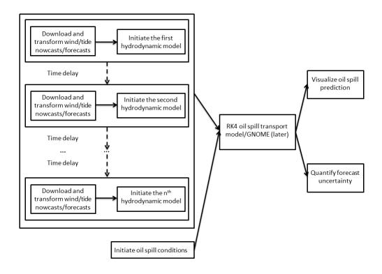
Figure 1.3.1: HyosPy wrapper structure (The big box on left represents a sequence of hydrodynamic models running with wind/tide force and pre-defined intervals marked as Time delay. The results of this model sequence along with the initial oil spill conditions are used to visualize oil spill predictions and quantify forecast uncertainty by using RK4 oil spill transport model.)
