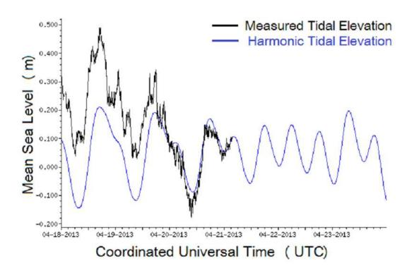
Figure 3.6.1: Typical measured and predicted tidal elevations (TCOON, 2013)
