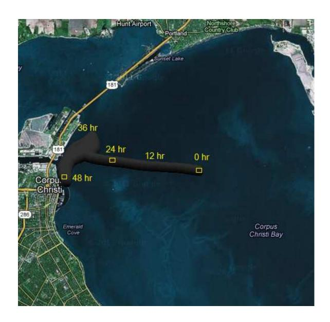
Figure 4.1.4: Oil spill trajectory prediction (48 hours). Results from 12 different RK4 surface tracer simulations plotted using Google Earth
