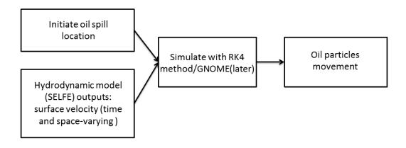
Figure 3.8.1: RK4 Surface Tracer Transport Routine Mechanism
