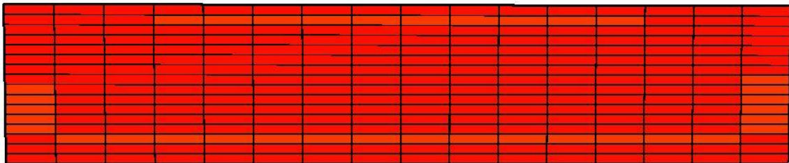
Water saturation inside fracture after 150 days
