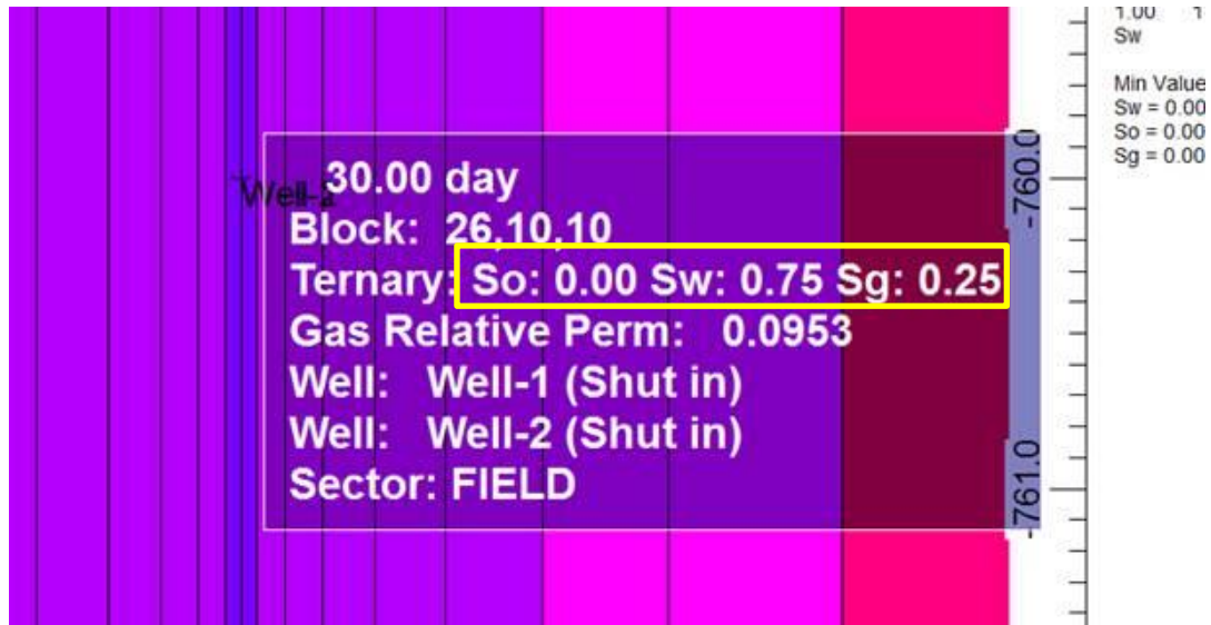
Figure 4.33: Water-Gas saturation near fracture after shut-in (VDRP OFF)
