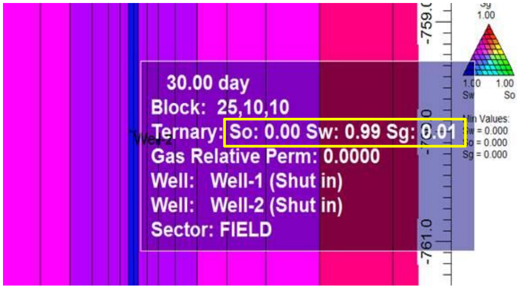
Figure 4.32: Water-Gas saturation near fracture after shut-in (VDRP active)
