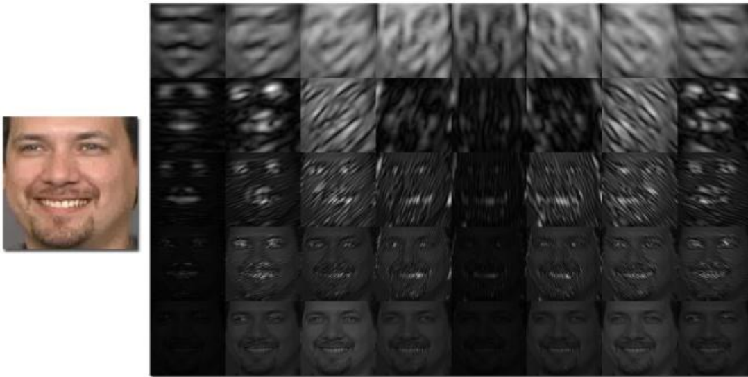
Figure 3.5: Original face image (left) and the set of output images of Gabor filter bank (right). The face image is from the Moving Faces and People dataset. It can be observed, from the figure, how the changes in orientation and wave-factor in the Gabor filter affect the response of the image.
