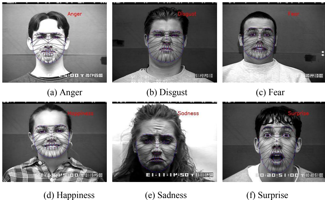
Figure 3.1: 68 landmarks that are used as characteristic points of the face shape of an expression. They are selected to lie on the contour of the eyebrows, eyes, nose, inner mouth lip, outer mouth lip, and chin.
