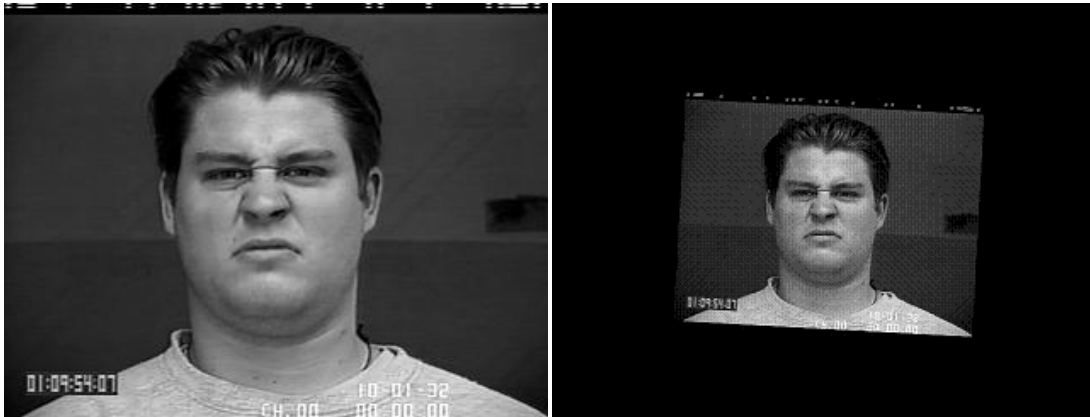
Figure 3.3: Example affine transformation result of a face image. The original image is scaled, shifted, and rotated so that the new face shape aligns to the optimally determined mean shape.
