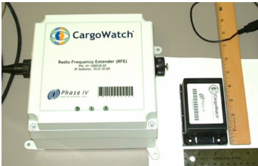
Figure 3.4: RFID reader and tag for the fixed system
