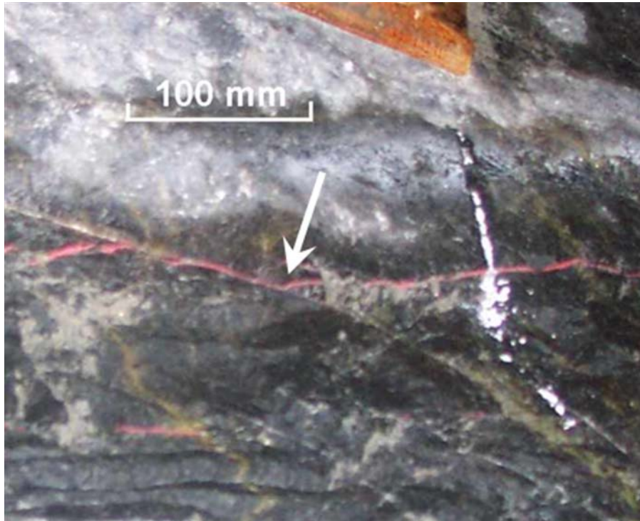
Figure 1.2: Part of the hydraulic fracture (red line) exposed by mining at Northparkes. Note offset as the fracture interacts with a cemented natural fracture (by Rob Jeffrey from CSIRO website). The hydraulic fracture propagated from right to the left. Offset (diversion) point is demonstrated by an arrow.
