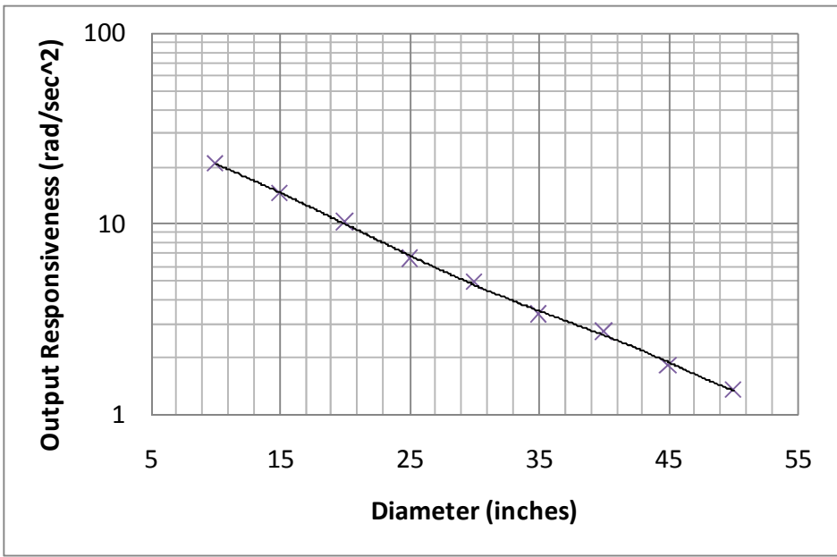
Figure 6.21: SRM+Star Compound+PEGT Output Responsiveness as a Function of Diameter
