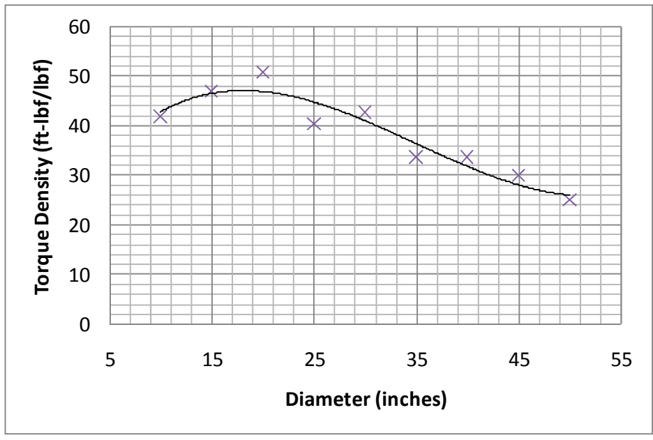
Figure 6.20: SRM+Star Compound+PEGT Torque Density as a Function of Diameter
