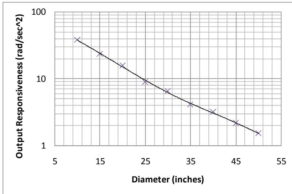
Figure 6.14: SRM+Star+PEGT Output Responsiveness as a Function of Diameter
