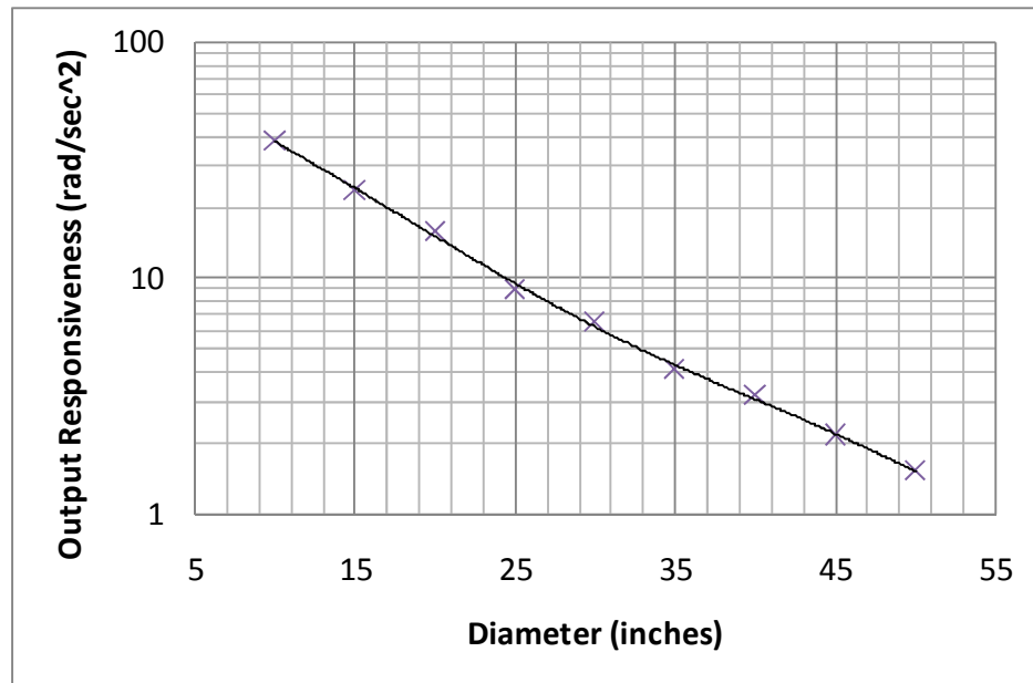
Figure 9.18: SRM+Star+PEGT Output Responsiveness as a Function of Diameter
