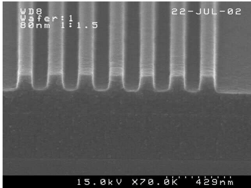
Figure 2.7 Dense 80 nm features printed with acrylate imprint resist.
