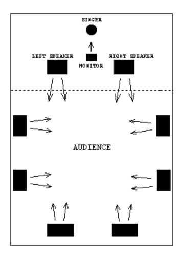
Figure 2: Example of eight-speaker sound diffusion system with singer.
