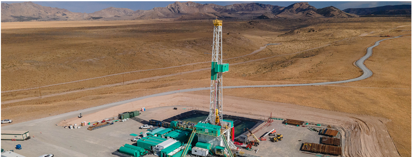
Figure. 1.9. Utah FORGE is an underground field laboratory sponsored by DOE for developing, testing, and accelerating EGS technologies. Source: FORGE, 2020a; 2020b.
