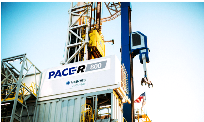
Figure 6.18. An example of oil and gas rig automation. In 2022, NABORS and ExxonMobil announced the oil and gas industry’s first fully automated land rig, which included a first of its kind robotics module. Rig floor automation may improve worker safety and process consistency in both the oil and gas, and geothermal contexts. Source: NABORS, 2022.
