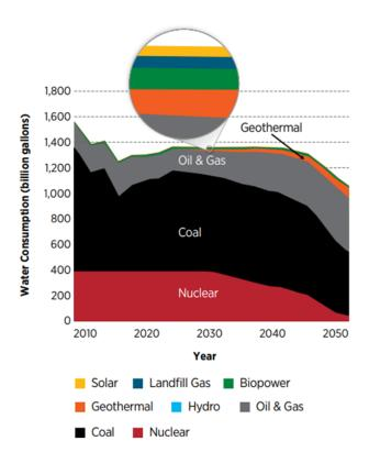
Figure 10.2. Water-consumption impacts from the geothermal power section in billions of gallons (1 gallon=3.8 liters) under the Technology Improvement scenario. Source: Adapted from Millstein, et al. (2019).
