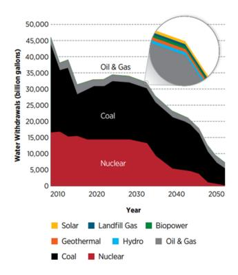
Figure 10.1. Power-sector water-withdrawal impacts in billions of gallons (1 gallon=3.8 liters). Source: Adapted from Millstein, et al. (2019).
