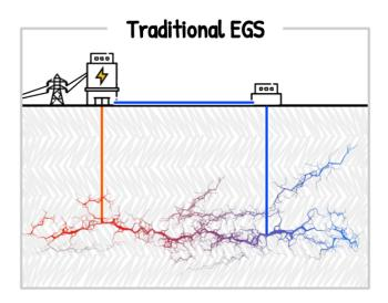
Figure 10.3. An open to reservoir geothermal system. Shown is a traditional EGS concept. Source: The Future of Geothermal in Texas, 2023.
