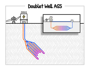
Figure 10.4. Example of a "Closed to Reservoir" AGS design. Source: Adapted from Eavor, 2021.
