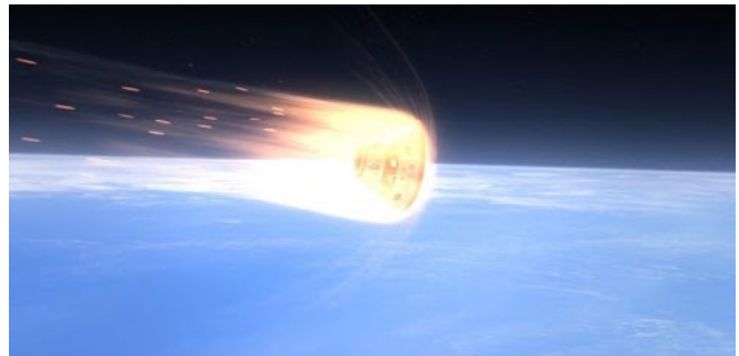
Figure 8.3. Artist rendering of an atmosphere reentry vehicle on descent. Skin temperatures on reentry vehicles as well as hypersonic aircraft can reach well over a thousand degrees. Source: NASA, 2022.
