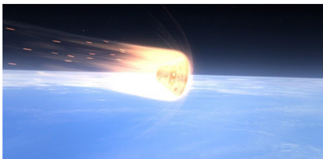
Figure 8.3. Artist rendering of an atmosphere reentry vehicle on descent. Skin temperatures on reentry vehicles as well as hypersonic aircraft can reach well over a thousand degrees. Source: NASA, 2022.
