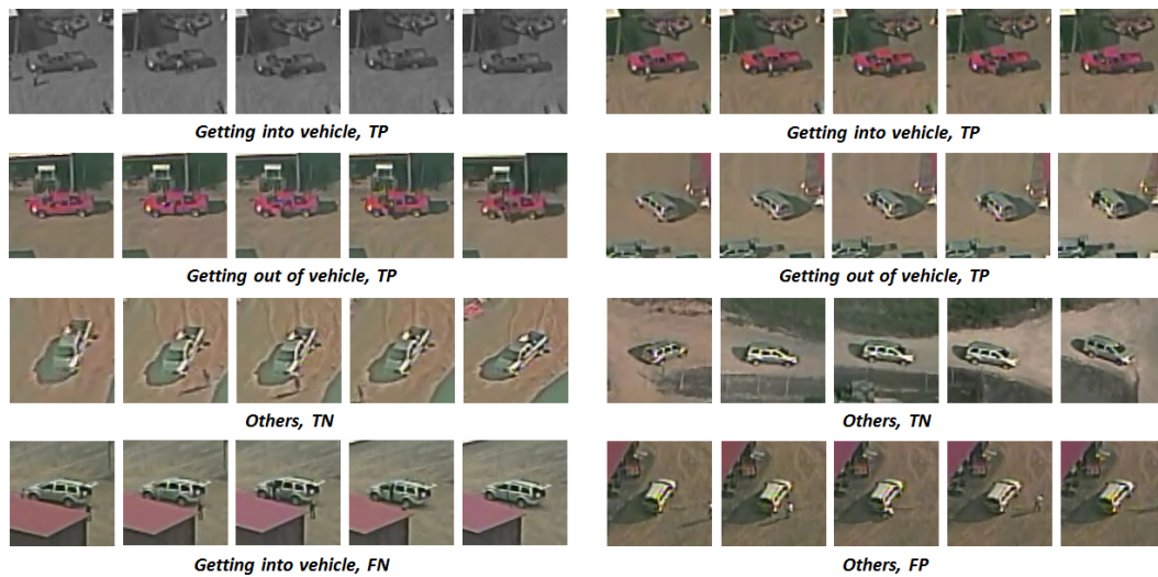
Fig. 5.8: The snapshots of four true positive (TP), two true negative (TN), one false negative (FN), and one false positive (FP) sequence are shown. We treat the subject human-vehicle interactions (getting into vehicle, getting out of vehicle) as the positive class and all other events (others) as the negative class.
