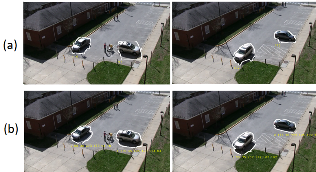
Fig. 4.5: (a) Vehicle detection using 2D templates from 3D vehicle models without shadow (b) Vehicle detection using 2D templates from 3D vehicle models with shadow.
