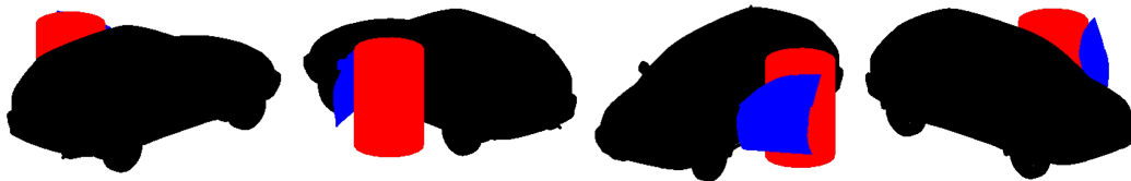
Fig. 3.4: Example occlusion types generated based on the simulation. Representative occlusion types describing relationships among human, door, and vehicle body are presented.
