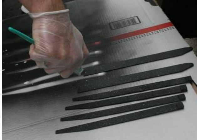
Figure 2.3: Application of a stochastic speckle pattern via the toothbrush method
