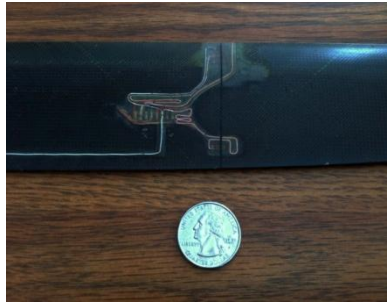
Figure 1.1: Strain gage mounted on a 0.15 scale Bell 412 helicopter blade
