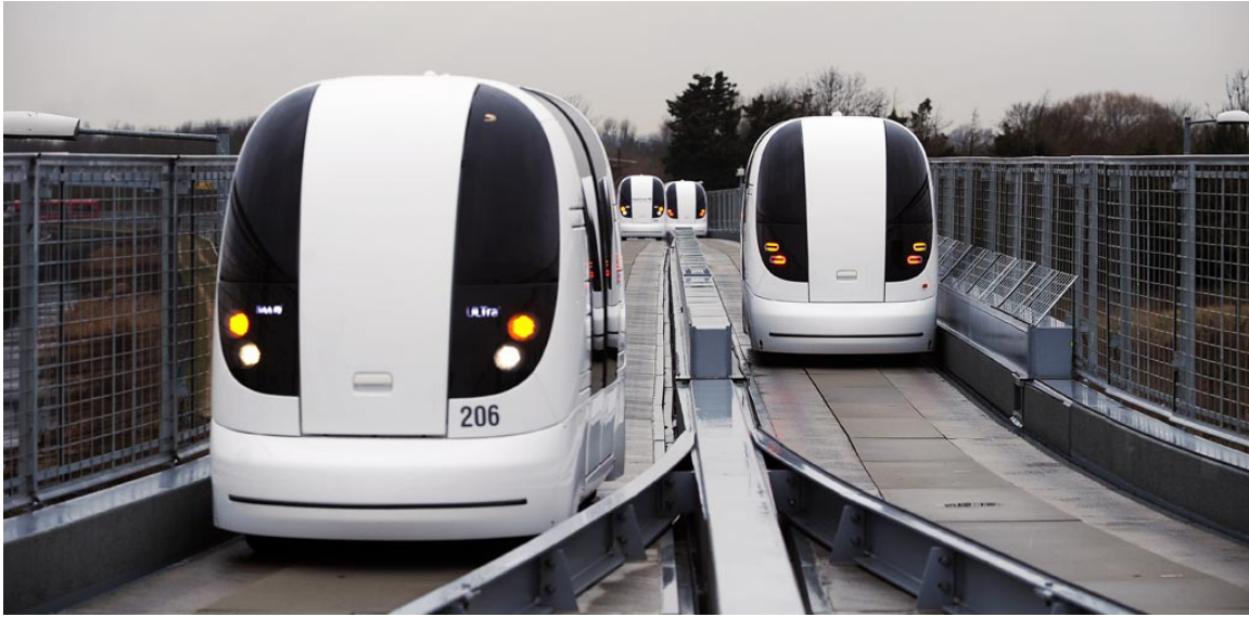
Figure 17: Personal rapid transport, ULtra, as used at London's Heathrow airport
