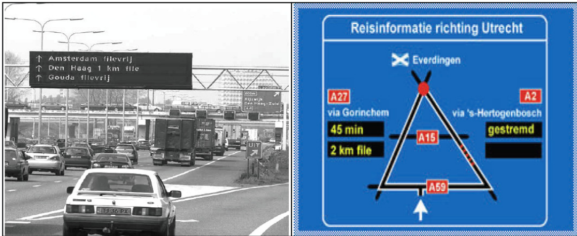
Figure 5: Example of a Dynamic Route Information Panel (DRIP) and a Graphic Route Information Panel (GRIP)
