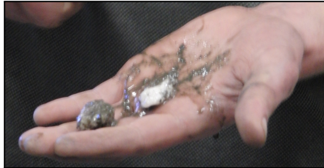
Figure A.5: Photograph of a methane hydrate sample used in the experiment described in Ch. 4. A significant percentage of mud content in the sample may have contributed to the discrepancy between tabulated properties of methane hydrates and results of the present experiment.
