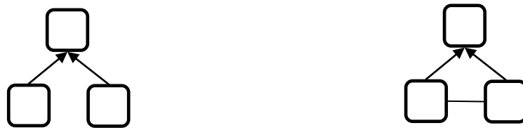
Figure 8.7 Parental Relationships without (left) and with (right) Common Design Parameters at the Subsystem Level
