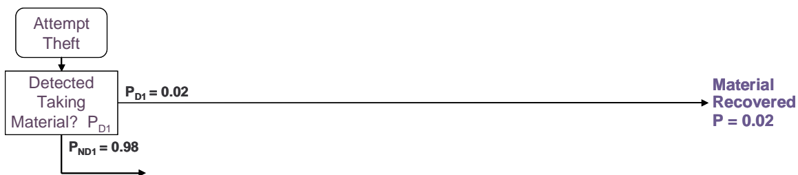
Figure 21: Event 1 of the ESD – Detection of the insider taking the material by the PPS in the MAA
