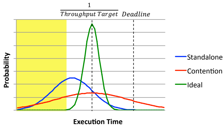
Figure 2.1: Example LC completion time probability density functions when run alone, under contention, and in an ideal scenario; the shaded region points to underutilized resources when run alone.
