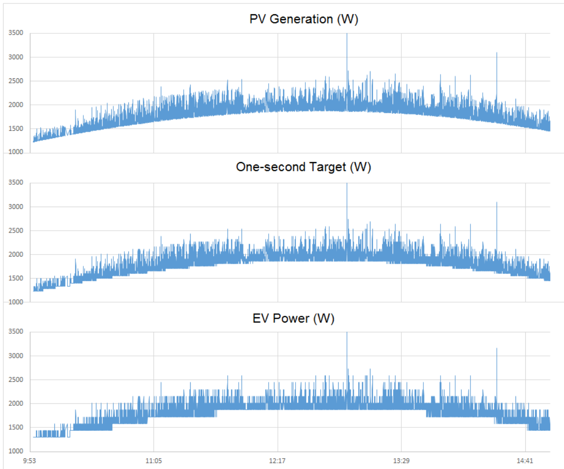
Figure 12: Local EVSE control charging an electric vehicle under a PV envelope
