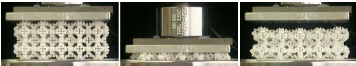
Figure 13- Compression of a helical strut sample
