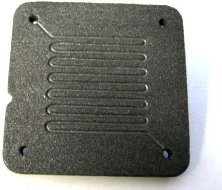
Fig 4(c). Brown part before infiltration (50mm by 50mm by 5mm)
