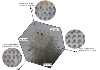
Figure 5 Manufacturing induced deformations in the cross section of the struts in the different building directions
