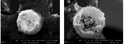
Figure 4 Cross-section of struts fabricated in the Z building direction (a) 0.6 mm, (b) 0.8 mm strut at P<sub>OI</sub>=10 W
