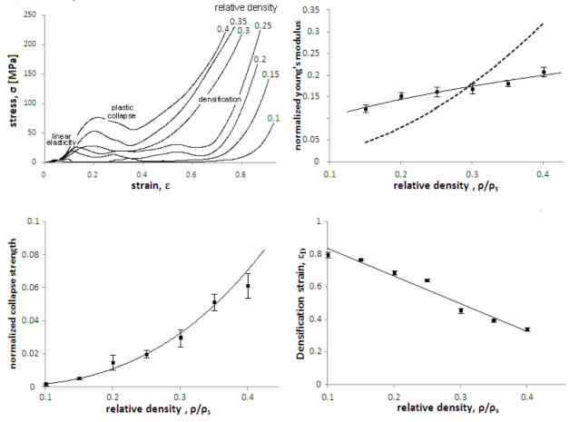
Figure 2 (a) Stress strain map for scaffolds manufactured by SLS, (b) relationship between the relative density and the normalized modulus (continous line – measured data, dotted line – Gibson-Ashby model), (c) relationship between the relative collapse strength and the relative density, (d) relationship between the densifications strain and the relative density of the scaffolds
