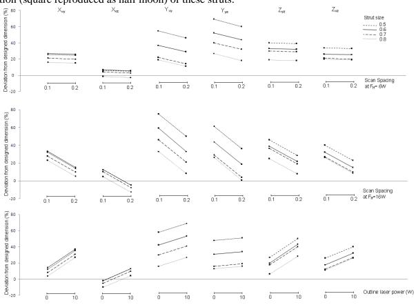
Figure 6 Process parameter effects on different strut sizes in different building and measuring directions, strut size range displayed is from 0.5 – 0.8 mm, target is being 0% of deviation
