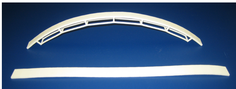
Figure 12. Arch prototype with and without lattice structure.
