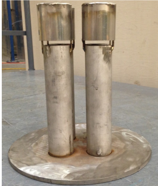
Figure B-2 – Total trapout tray placed at the top of the wall
