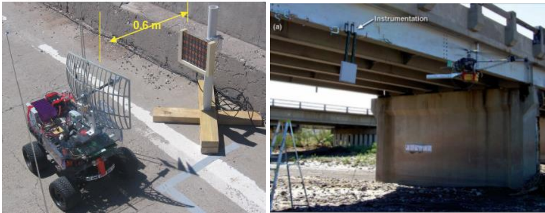
Figure 10: (left) From [40] terrestrial MA with instrumented bolt Wireless Impedance Device (WID) sensor node (right) From [41] Aerial MA with strain sensor WID.
