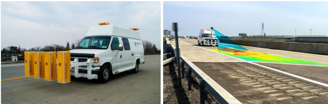
Figure 3: From [9] GPR (left) and IR thermal camera (right) used here to detect internal defects such as delamination in concrete caused from corrosion of embedded steel reinforcement bars.
