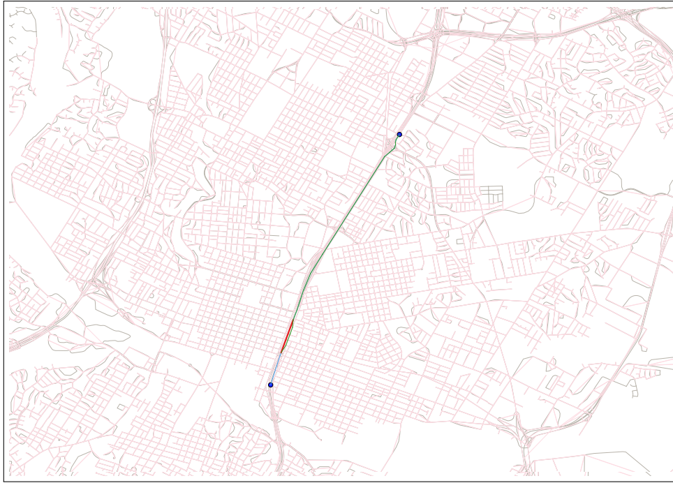
Figure 2.13: Optimal single route adjustment policy: Red solid line represents the optimal adjustment edge. Blue and green lines represent the non-adjusted and the adjusted shortest route respectively.
