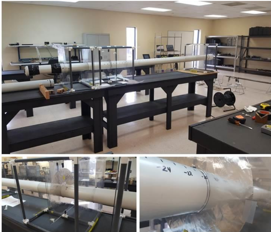
Figure 3.9: Laboratory experimental setup: top picture shows main set-up which allows moving fracture models across the center of receivers; during the tests, the surrounding of the tool was kept free of metal; bottom-left picture shows the plastic box which keeps fracture model in a given orientation; and bottom-right picture shows centralization of the fracture model with respect to the outer shell of the tool.
