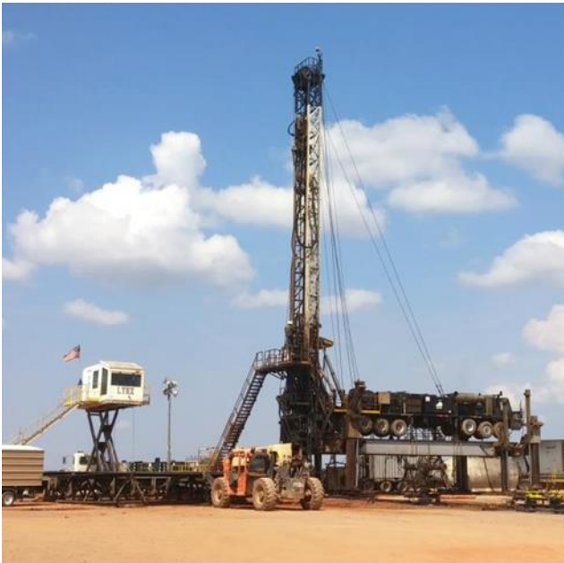
Figure 11. Superior mechanized, standalone snubbing unit.
