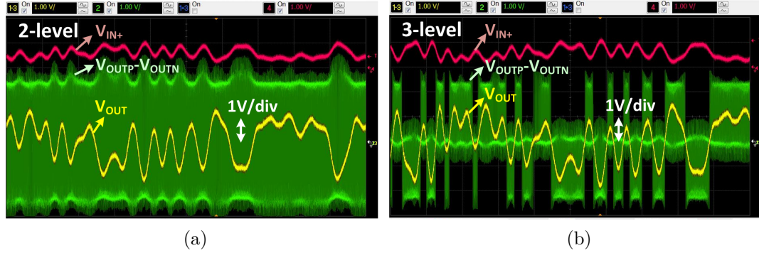
Figure 3.21: Measured waveform of 2/3-level PA operation with D8PSK modulation at f_{SW} = 60 MHz. (a) 2-level PA. (b) 3-level PA.
