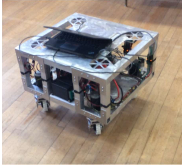
Figure 6-3: The NRG's holonomic platform with four actuated-caster swerve steer wheels.
