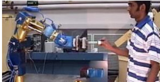
Figure 2.1. A force-based teaching HRI application implemented on an off-the-shelf modular manipulator from Amtec, Germany. An admittance-type control was implemented using a 6-axis end-point force/torque sensor from ATI. The OSCAR (Kapoor and Tesar, 1996) manipulation software enabled extending this application to multiple robot platforms.
